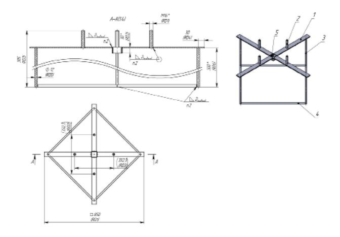
The base is to be filled with concrete. The ground at the place of installation of the charging station must provide high stability of the base. There should be no underground cables or pipes in the area around the foundation.
